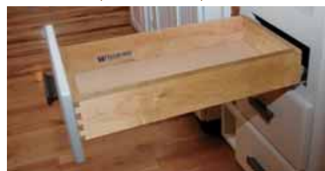
3/4" Solid hardwood drawer box in natural finish with classic dovetail construction and undermount full extension soft close drawer slides with Blumotion
